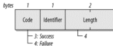
Figure 6-4. EAP Success and Failure frames
